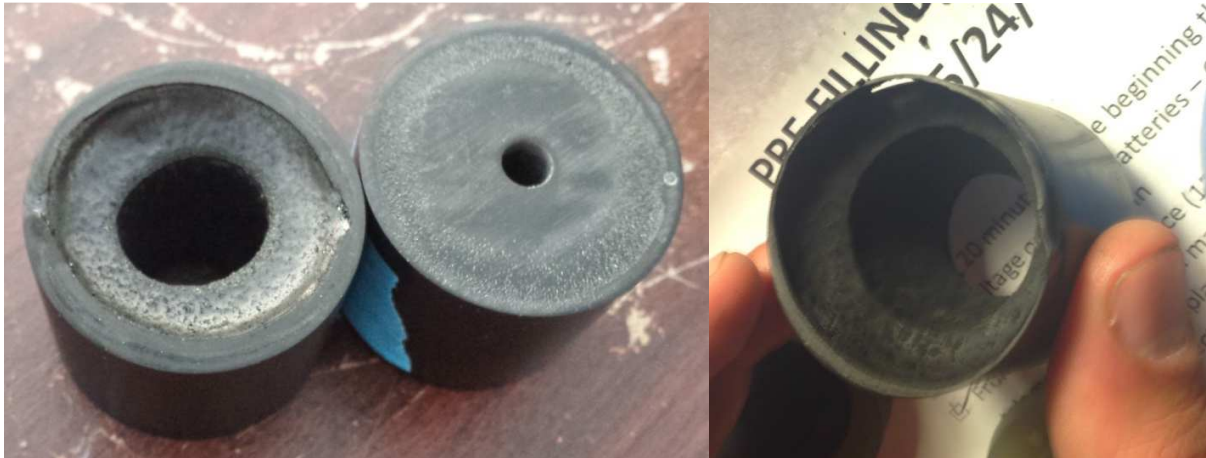
Figure 15: Recirculation driven end burning in hotfires 1 (left) and 2 (right).
